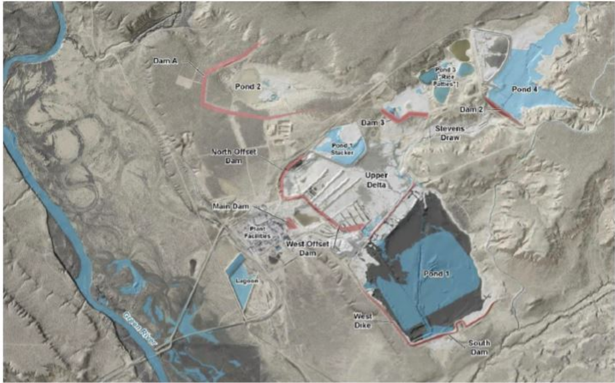
Source: Barr- Ciner-2020_Dam-Safety-Report_20210224-signed.pdf Figure 17.1 Siseecam Tailings Impoundments and Evaporative Ponds
