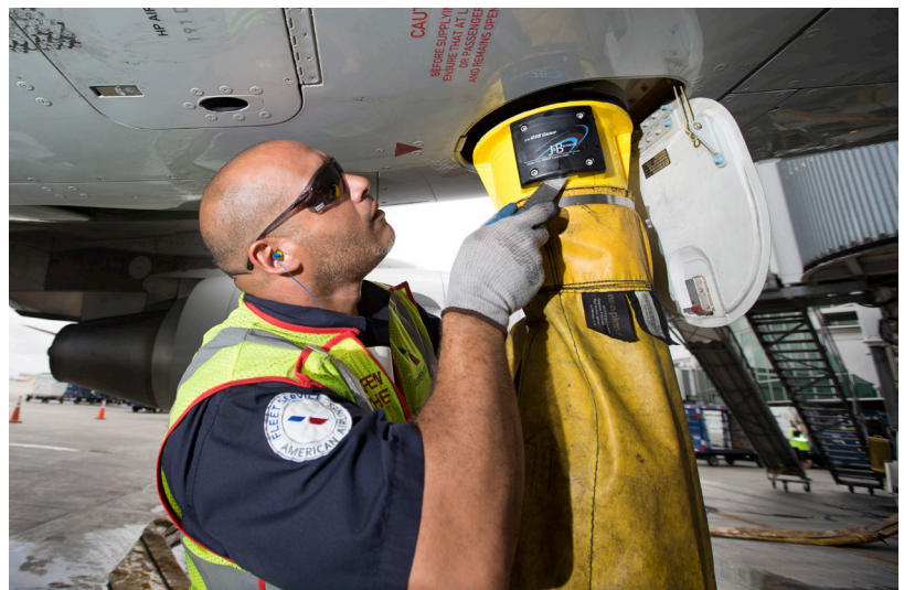
Miami International Airport Fleet Service team member Wilfredo Rodriguez-Garcia helps reduce aircraft fuel consumption by using pre-conditioned air from the ground.
