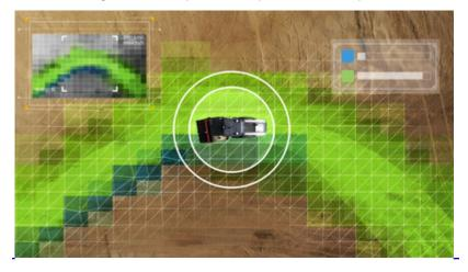
The field study compared fuel burned, pass count and total time required to complete a compaction operation performed manually and using the Horizontal Steering Control functionality for Trimble<sup>®</sup> Earthworks Grade Control Platform for Soil Compactors. Trimble Earthworks Horizontal Steering Control automatically steers a soil compactor using a 3D model or compaction pass line, which helps to improve compaction productivity and quality by precisely controlling overlap between passes.
