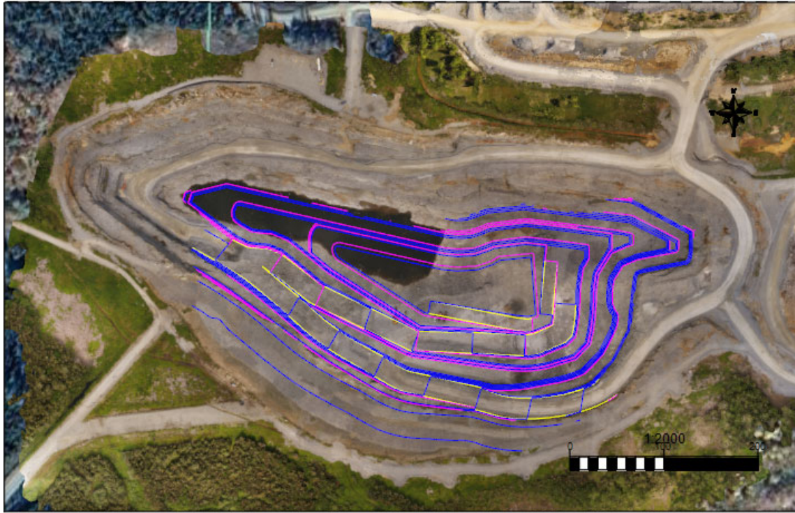
Figure 16-8: Final Pit Layout Plan, Grand Duc
