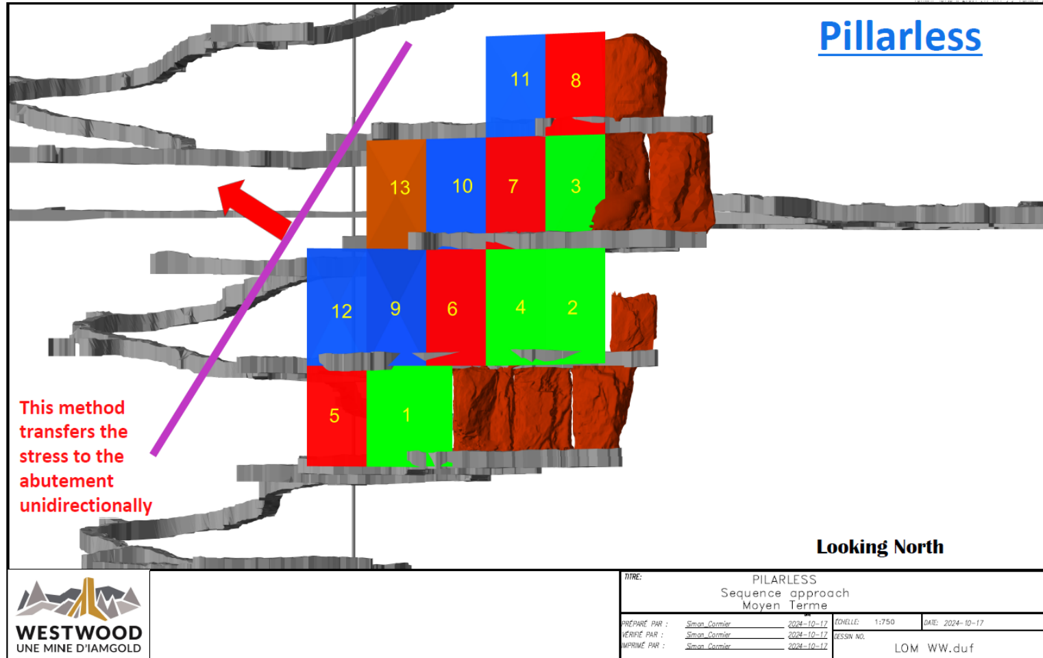
Figure 16-4: Current Mining Method, Westwood
