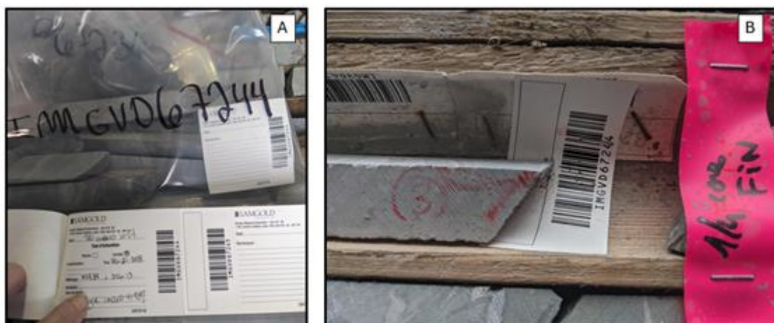
Figure 12.4 – Photograph of core resampled by InnovExplo: (A) method for sample identification; (B) remaining quarter-core witness samples. Hole ML-21-258.
