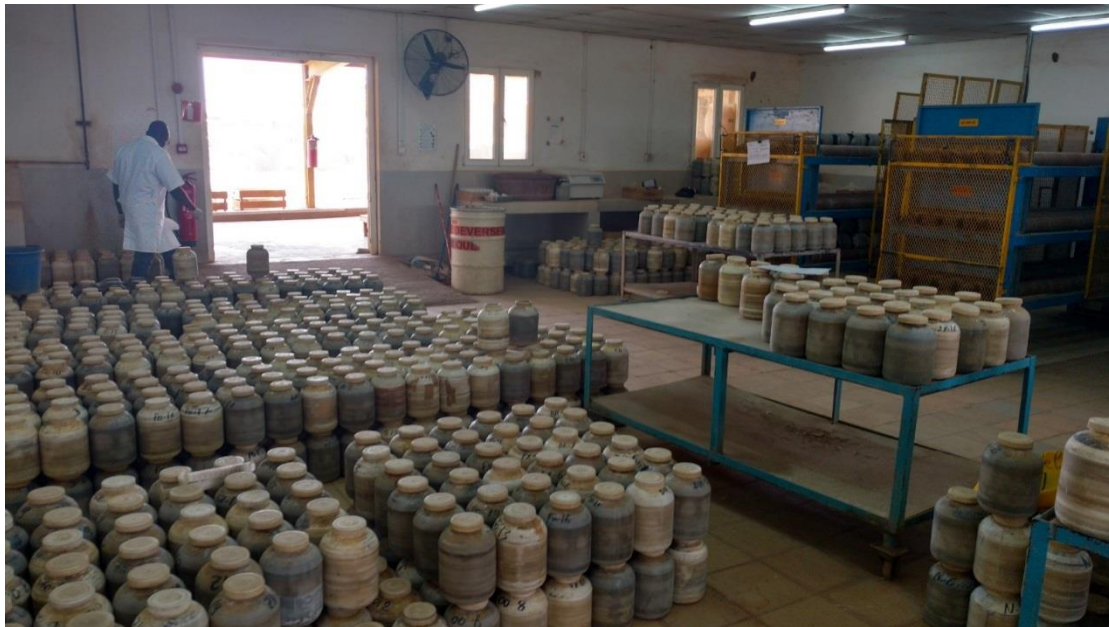
Figure 11.4: Leachwell Samples During the Leaching Process. Note Batches of 24 on the Racks
