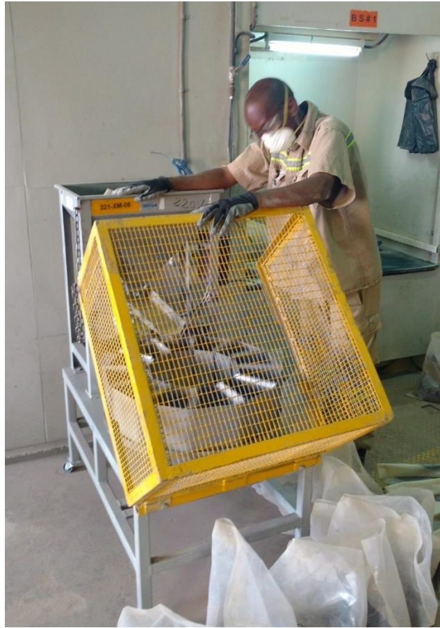
Figure 11.3: Rotary Splitter in Operation
