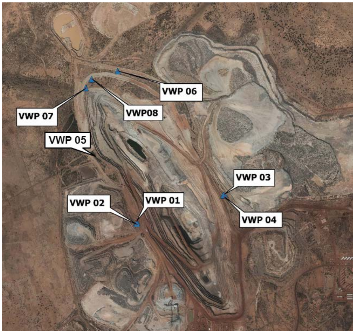
FIGURE 16-6 LOCATION OF THE ESSAKANE PIT VWP
