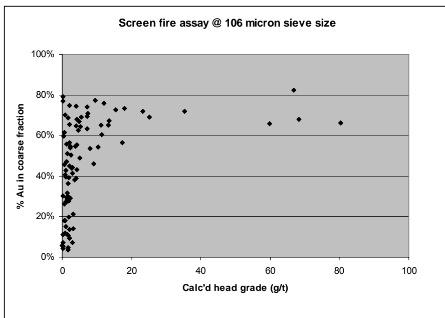
Figure 9.5 Screen fire assay results for 96 x 1kg pulverized samples
