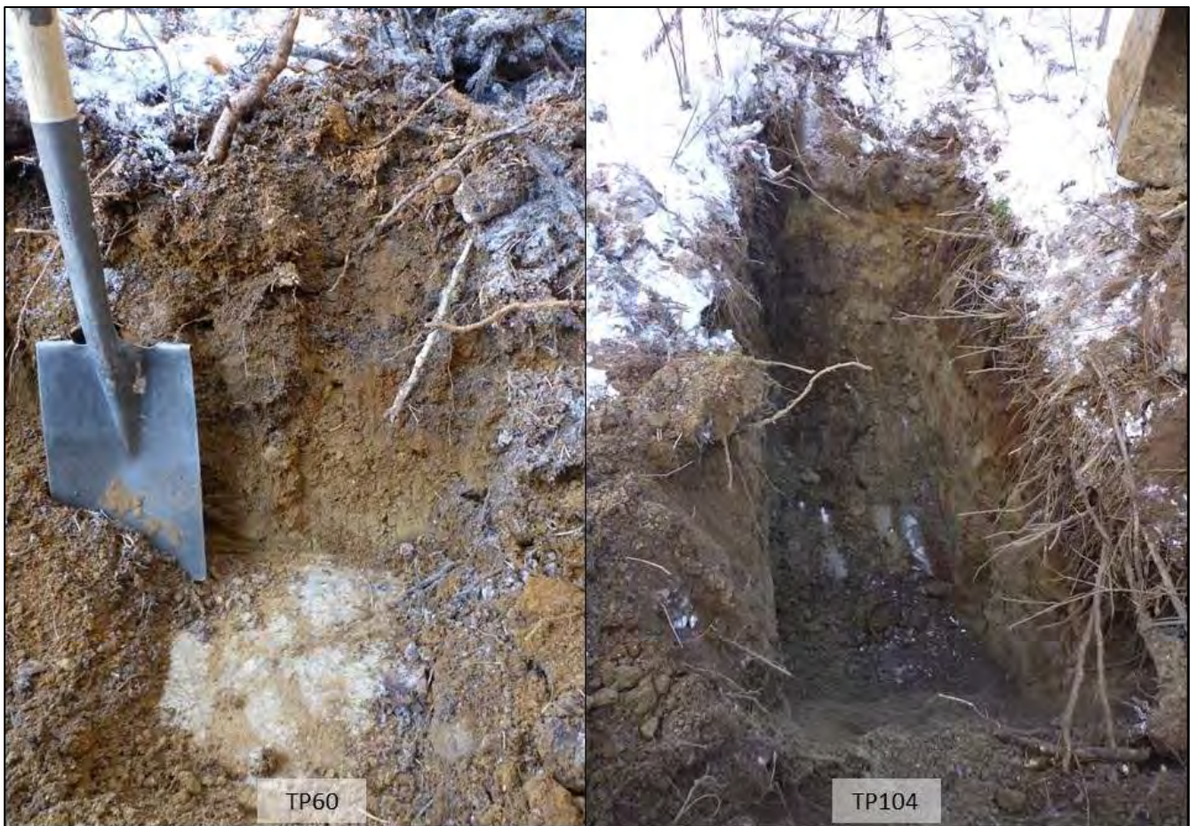
Photograph 3: Typical overburden stratigraphy at higher elevations; showing bedrock exposed in the bottom of the test pit.
