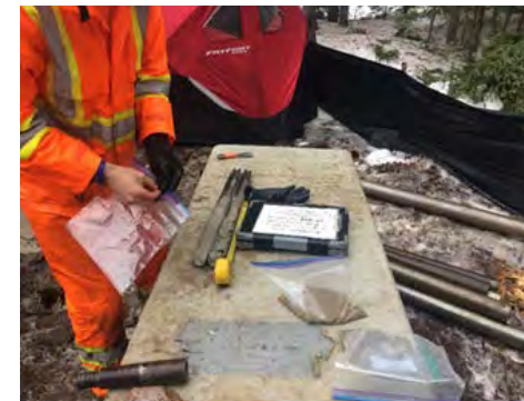
Drilling Program for geotechnical Investigation – split spoon sampling
