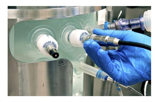
Above: The Mettler-Toledo InSUS 310i is the first digital single-use pH sensor for use in bioprocessing. An integrated memory chip stores relevant sensor and factory calibration data and enables immediate measurement without manual configuration. Intelligent Sensor Management (ISM) features are accessible when paired with the digital InSUS H30i sensor head. The gamma and X-ray resistant pH sensor is designed for integration into single-use process bags and have a 30 month shelf life.
