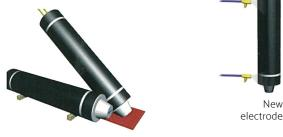
Clean both the socket of the old column and the body, pin and end face of the new electrode with an airline.
