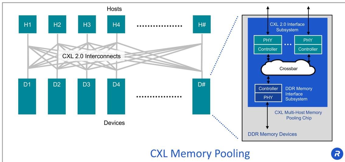
Pooling provides additional main memory to Hosts on an "as needed" basis, improving performance, efficiency and TCO. Pooling ultimately supports disaggregation and composability.
