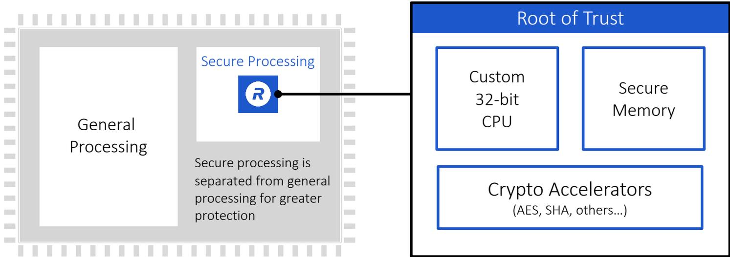
Secure Co-Processor Root of Trust (RT-600 Series)
