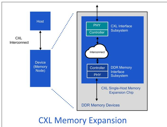
Expansion provides more main memory to Host (CPU) for higher performance on high-capacity workloads
